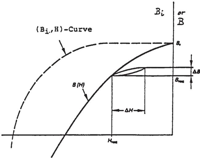
FIG. 3 Normal and Intrinsic Demagnetization Curves with Symbols for Special Points of Interest and Definition of Salient Properties. Illustration of Recoil Loop. Recoil Permeability is Defined as  $\mu_{rec} \Delta B / \Delta H$
